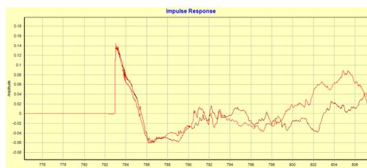
Looks good. No pre-ringing at the beginning of the vertical step with no discontinuities in the vertical step, meaning that all frequencies are arriving at ones ears at the same time. This is much closer to an ideal speaker’s step response and a major improvement over the measured step response in the previous “Filter the measurement” section. For a refresher on what an ideal speaker’s step response should look like, scroll to section “[Time Coherence – Step Response](#)”
