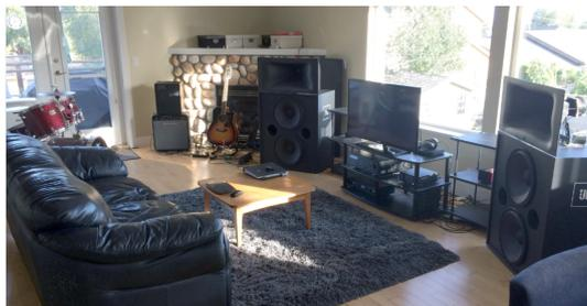
I love high efficiency loudspeakers for their perceived dynamics. These 2-way [JBL 4722 cinema loudspeakers](#) are about as sensitive as one can get, rated at 104 dB SPL at 2.83 volts at one meter. I selected the biamp version and performed a [compression driver upgrade](#), as suggested by user notnyt on the AVSforum. The 4722's are fugly looking, but sound huge. Note one can use Audiolense with any passive speaker or virtually any loudspeaker for that matter, including surround sound systems.
