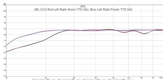
One can see the left and right pair's frequency response is virtually identical. Overlaying the same measures, but change the view to group delay:
