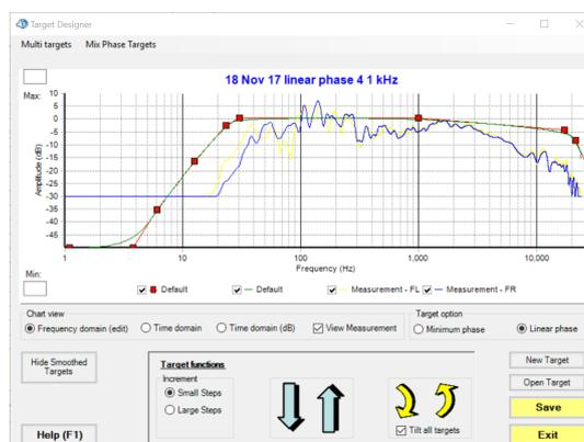
Small variations in targets will impart a certain perceived timbre or tone quality. The tilting target, before this one, will have a bit of a recessed midrange, whereas flat to 1 kHz, the midrange will be a bit more out front. Again, worth creating a few targets and switching between to determine ones preference. For the purpose of this article, I went with the tilted target, but later listened to the flat to 1 kHz linear phase target.
