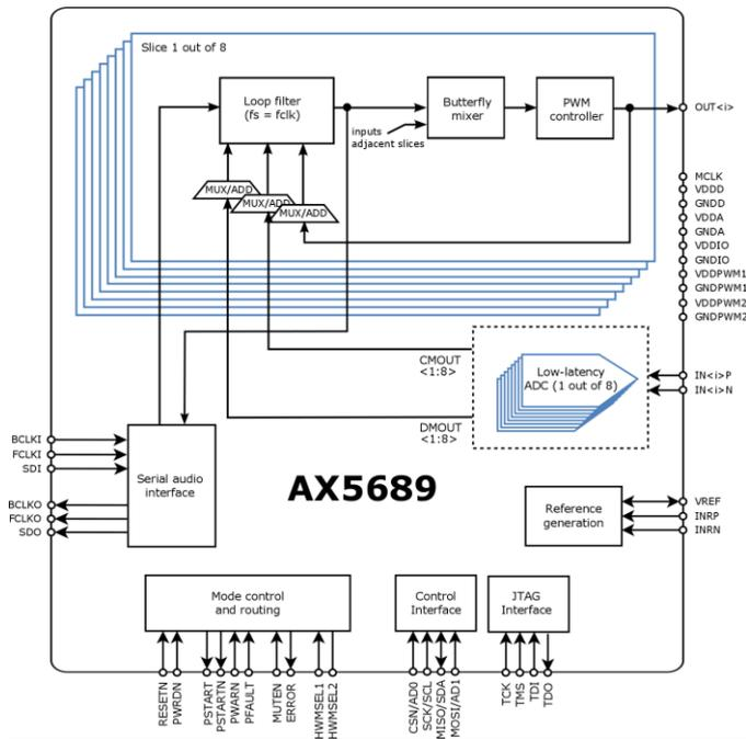
Figure 1 - AX5689 block diagram
