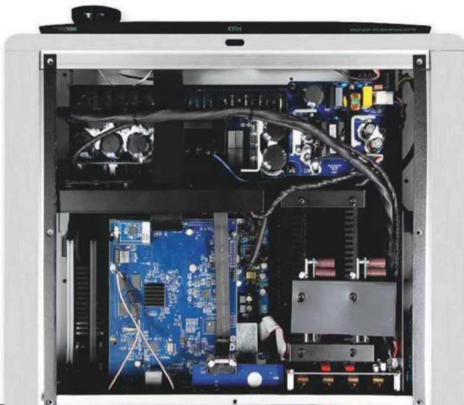
RIGHT: Substantial switchmode power supplies occupy the front of the amplifier [top], with network/Bluetooth, digital input and analogue (ADC) processing [lower left] and two of Purifi's Eigentakt Class D amplifiers [lower right]
