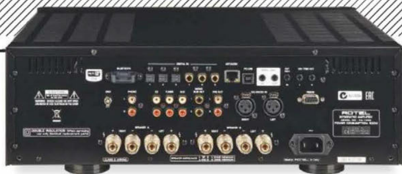
ABOVE: Four line (one on XLR) and MM ins are joined by sub and preamp outs plus pairs of switched 4mm speaker cable terminals. Digital ins include Bluetooth, S/PDIF (three optical, three coax) and asynchronous USB. Note RS232 and Ethernet IP control
