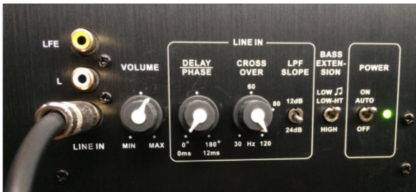
I am letting Audiolense take control of adjusting delay/phase and XO duties for the best possible integration with the rest of the drivers. I level matched the subs to the mains with the volume control.
