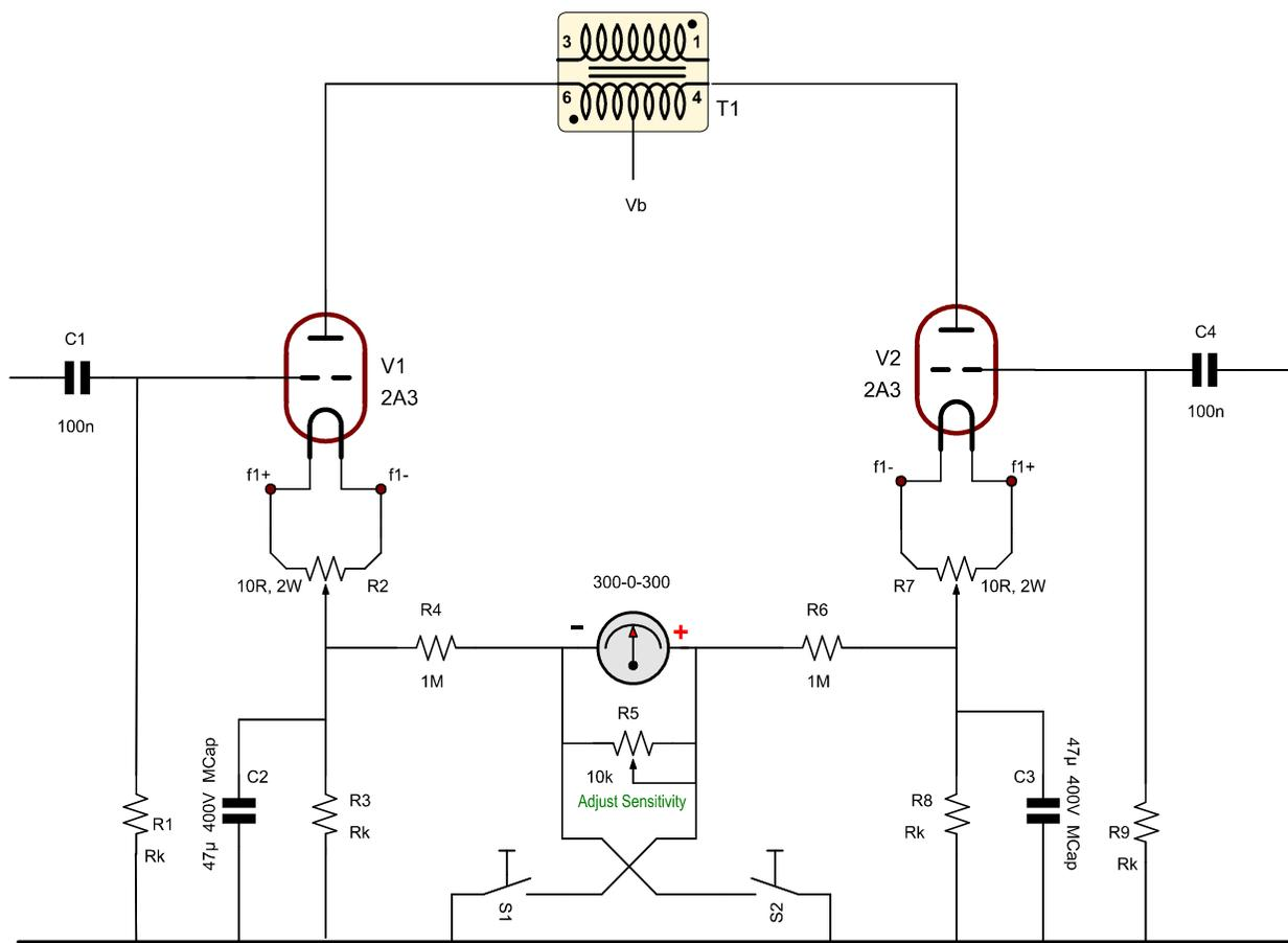
Push button for Bias Test of left tube. Needle moves to left
